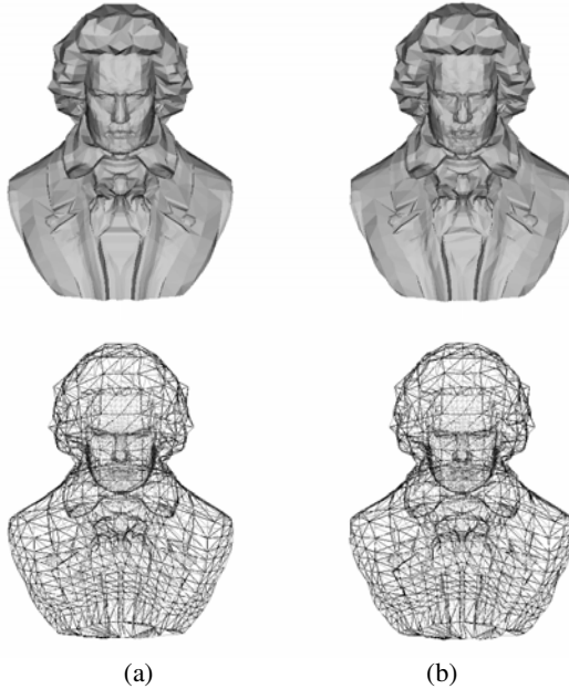
Fig. 5. (a) cover mesh model (b) stego mesh model : H(\mathbf{V}, \mathbf{V}') = 0.004415, DR = 1.0
